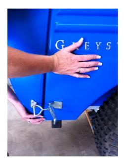
This photo shows how to seat the door before clamping – simply push in on the side wall while pulling the bottom of the rear door upward.
